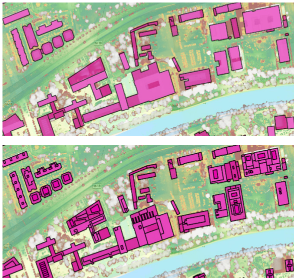
Figure 4 Segmentation of the building footprints to enhance the LOD. Source: Authors, 2025.
